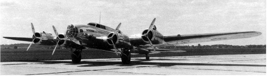
Boeing Model 299, prototype of the B-17 Flying Fortress. It could fly 250 mph at 14,000 feet and operate at 30,000 feet.
