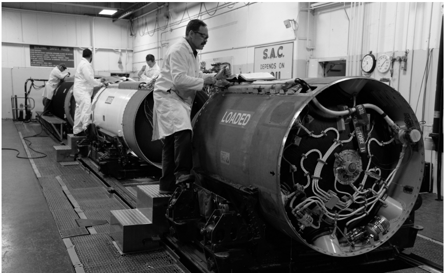
Technicians from the 309th Missile Maintenance Group perform planned depot maintenance on the LGM-30 Minuteman III ICBM in 2016.
